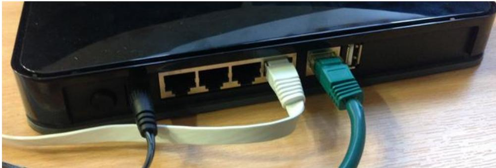
Please connect an Ethernet cable between port 1 on the back of the Netgear and your computer.
