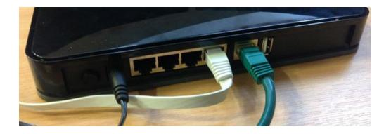
Please connect an Ethernet cable between port 1 on the back of the Netgear and your computer.
